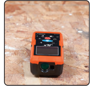
Cal3: Rotate 180°, LCD towards you.
